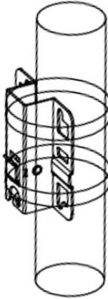
Figure 3-3 Mounting the Plate on a Pole
